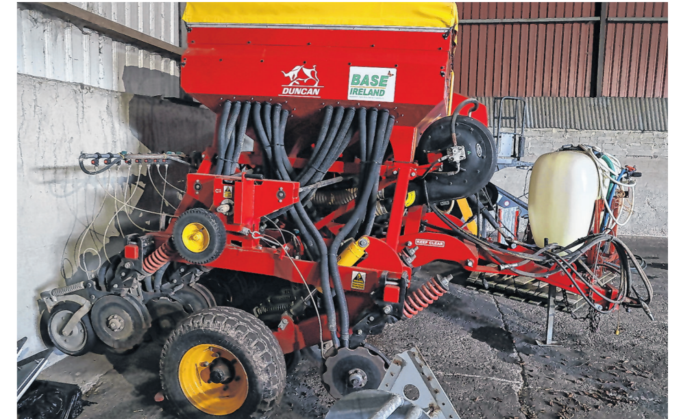
Tom's Duncan Enviro DD30/35, a double disc air seeder
