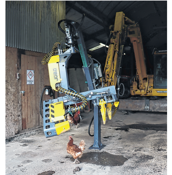
This Finland-built Syketec JOBO 55 harvester allows Tom to thin his forest without relying on a contractor
